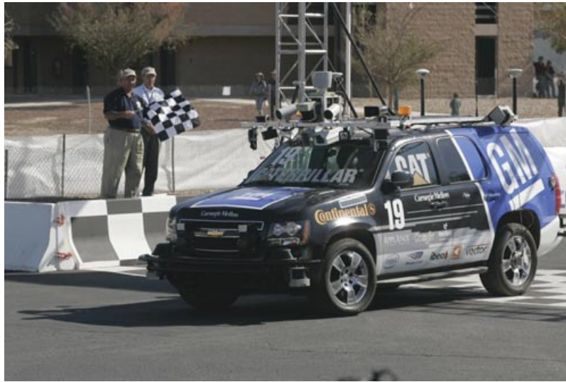
Figure 1. Boss, the autonomous Chevy Tahoe that won the 2007 DARPA Urban Challenge.
