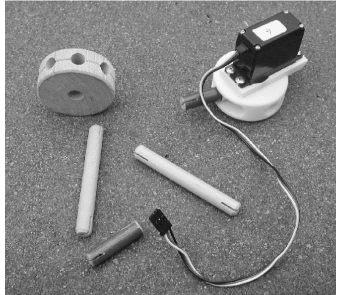
Fig. 2. Basic building blocks of the system: bars of regular lengths and fixes or actuated joints.
