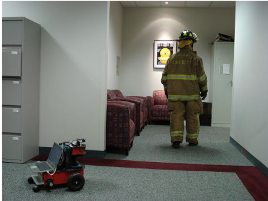
Figure 4.7: Volunteer firefighter searching with a Pioneer mobile robot. The robot and humans execute a schedule that clears the environment of any worst-case adversarial target. The decentralized GSST algorithm allows the robot and humans to fill the necessary search roles. The agents share their paths and a spanning tree that guides the search.
