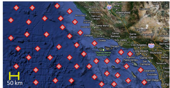
Fig. 1. Example sensor deployment on the ocean floor to monitor environmental conditions. Such sensors remain in place for many months. Retrieving data from the sensors during deployment is challenging due to communication limitations underwater. A mobile AUV equipped with an acoustic modem can act as a data collection device in this scenario by traversing a path that minimizes travel time and maximizes information gathered.
